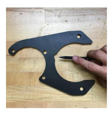
Before installing the brackets, locate the notch as indicated. This will be mounted **UP** when the bracket is installed on the axle. Once installed, the brackets will position both calipers to the **REAR** of the axle.
