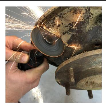
The brackets in this kit are designed to be installed without removing the differential cover. This can be done by use of a cut-off wheel or reciprocating saw to split the drum backing plate into two pieces for removal. If you wish to retain your drum backing plates, the axles can be removed from the housing by draining the fluid, then removing the differential cover, cross pin, and C-clip retainers.
