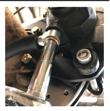
Install the banjo bolt and crush washers onto the hose as shown. If your hose has an offset, place the offset side of the fitting **away** from the caliper. Then install the hose onto the caliper as shown.
