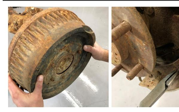
This installation refers to the **passenger side** of the axle. All steps are to be repeated on the driver side. Start by removing the factory drum. It may be necessary use a lubricant around the axle register to do this. Once the drum is removed, remove the brake shoe retaining springs (2 places) as shown.
