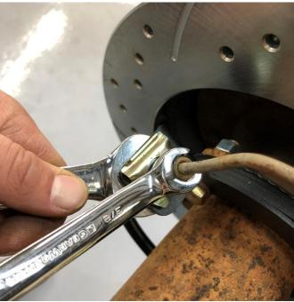
Install the retaining clip as shown, being careful not to bend the hose bracket. The factory brake line can then be repositioned into the top side of the brake line bracket and hose. **Use caution as to not kink the hardline during repositioning.** Next, tighten the brake line nut into your hose. It is best to use a wrench to support the rubber hose from spinning in the key of the hose bracket. **For kits without parking brake calipers, skip to Additional Information and Recommendations.**
